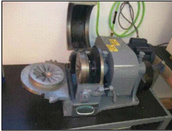
Figure 14: Mechanical Concrete Pulverization Machine and pulverized concrete sample
