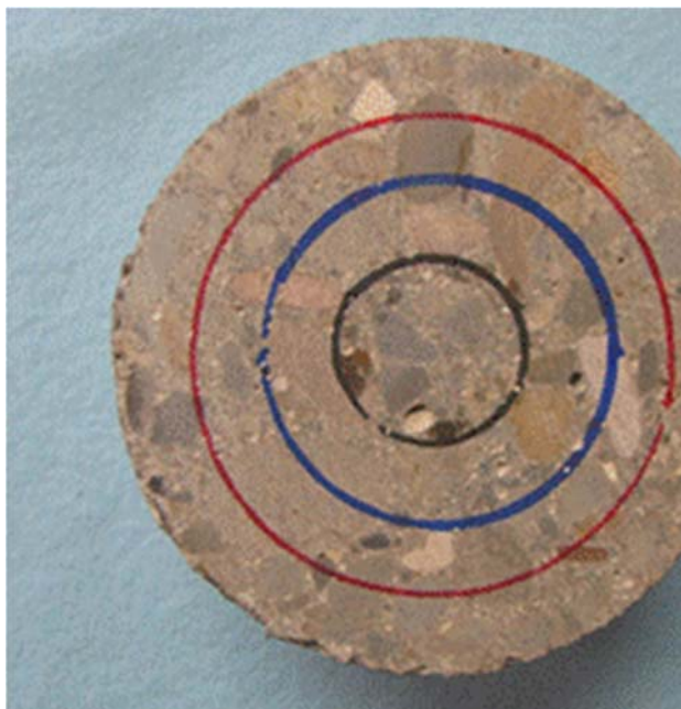
Figure 6: 4 Inch Core with 1 Inch Cross-Section Rings.
